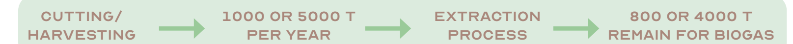
Figure 2: Diagram illustrating the process from harvesting to the production of extraction residues for biogas
